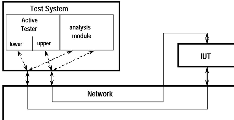
Fig. 3 - "Ferry" or "astride" test architecture.
