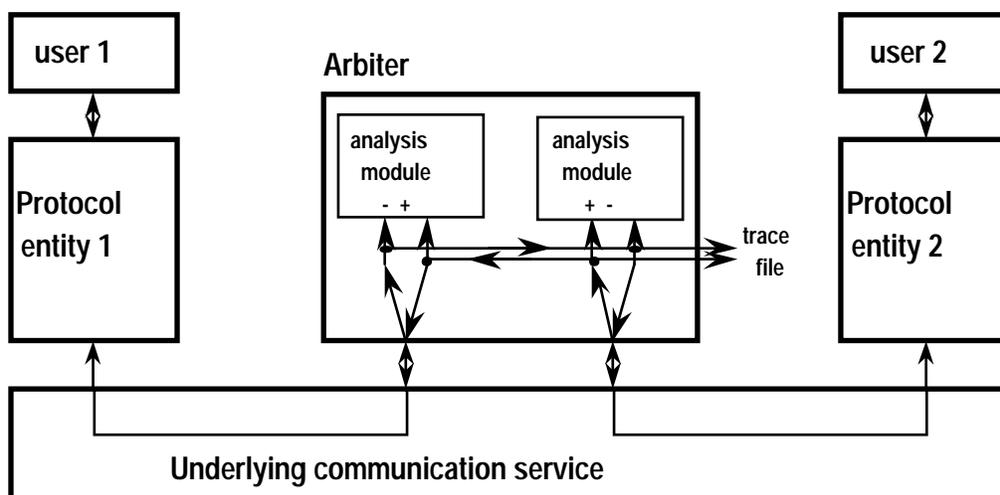
Fig. 2 - Test architecture with arbiter.
