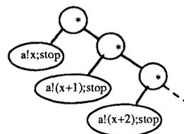
Figure 6: The activity tree of P[a](x:int):=(a!x;stop) \* P[a](x+1), where \* is one of the operators [], ||, ||| or > etc.
