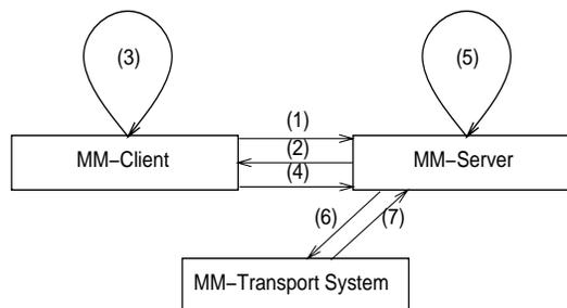
Figure 7. Variant II of QoS negotiation protocols.
