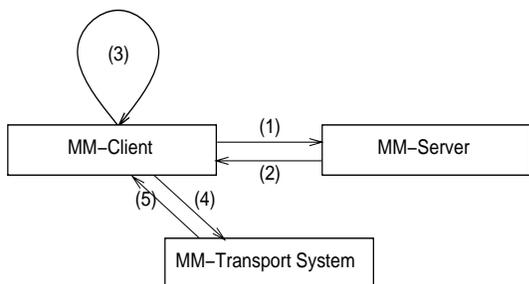
Figure 6. Variant I of QoS negotiation protocols.
