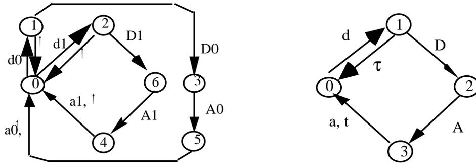
Fig.10 The modified channel specification with constraints: Chab' and Chns'.
