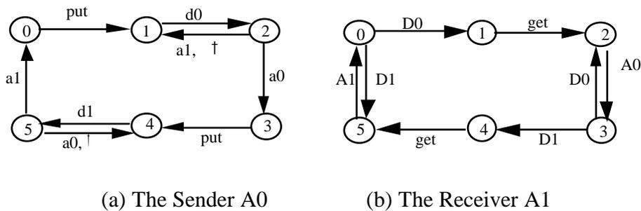
Fig.5 The AB protocol specification
