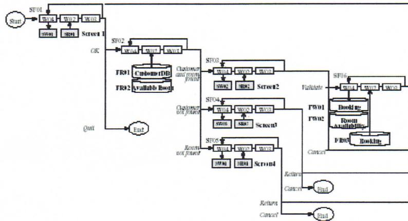
Figure 9 (from [Sali 01]): Process Route Diagram of the Room Booking example
