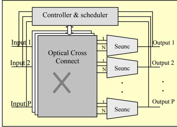
Figure 1 – Switch Architecture
