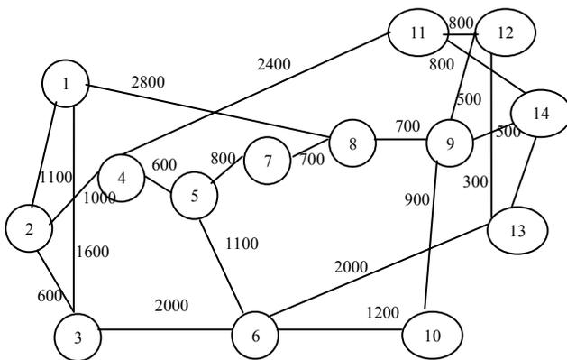
Figure 5 - NSFNET topology with 14 nodes
