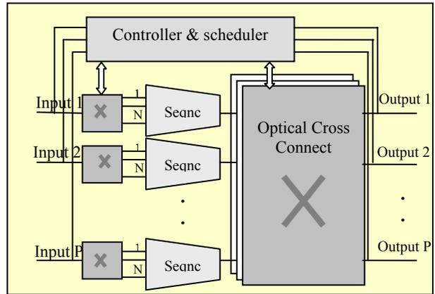
Figure 3 – Alternative Switch Architecture
