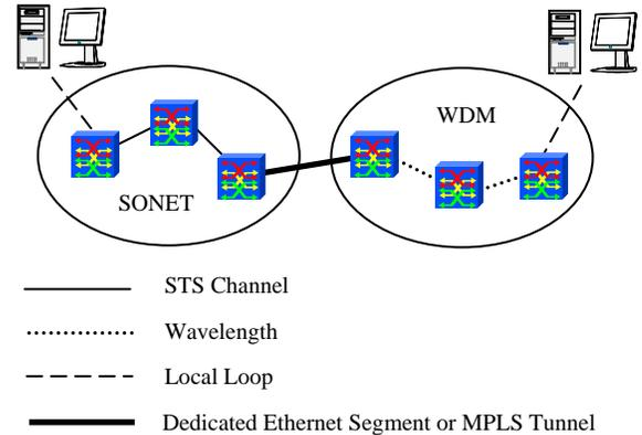
Fig.1 An E2e Connection Across Heterogeneous Domains
