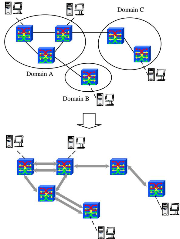
Fig. 4 A Layer 1 VPN Constructed With LP-WSs Acquired From Multiple Domains
