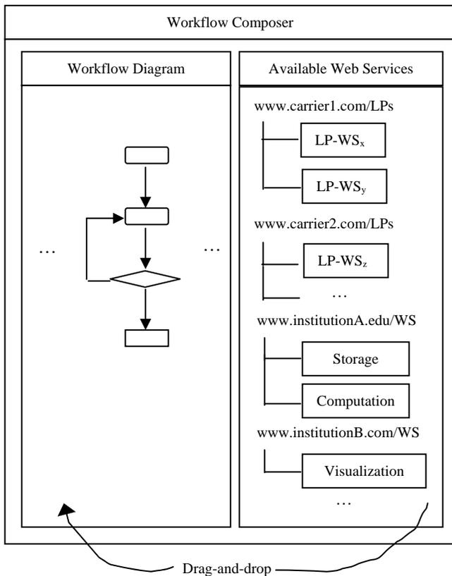
Fig. 5 Graphical Workflow Composer
