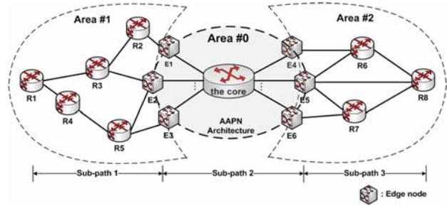
(a) Directly deploying AAPN as backbone area
