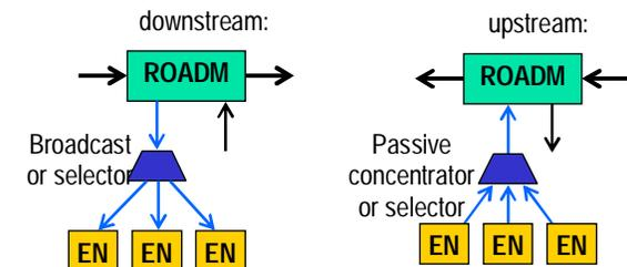
Figure 5. Deployment of concentrators and selectors separate from the RON.
