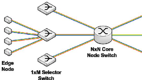
**Figure 3. Use of selectors in AAPN to allow for large numbers of edge nodes (image from [3]).**
