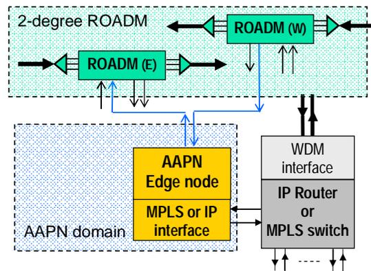
Figure 8. Agile edge node deployment attached to a 2-degree ROADM of the RON.
