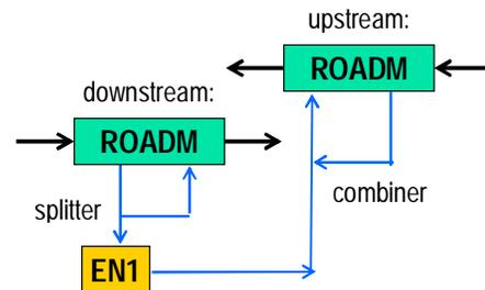
**Figure 9. Agile edge node deployment attached to a 2-degree ROADM when the WDM path/ring is used as selector/concentrator.**
