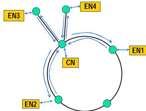
Figure 4. A five-ray star deployed on top of two ring networks (or a ring and two any other fibre links).
