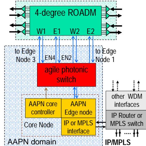
Figure 7. Agile switch and core node deployment attached to a 4-degree ROADM of the RON.
