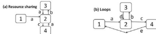
Fig. 2. (a) Fair resource sharing among states 3 and 4. (b) Program with embedded loops.
