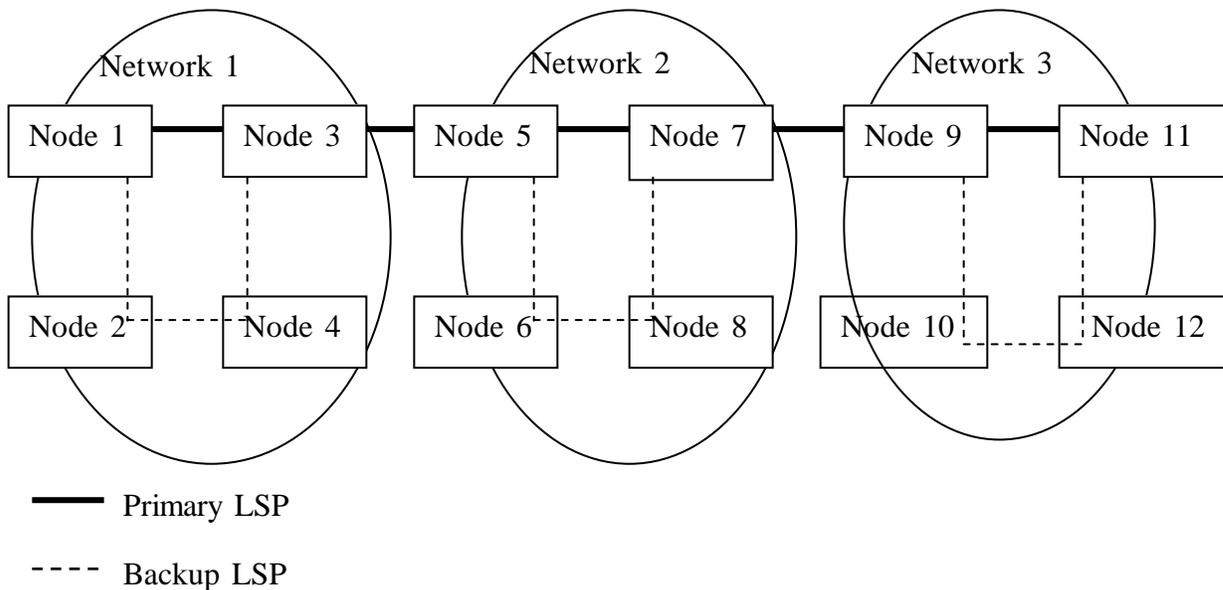
Figure 5.5: The logical view of the subnetwork protection
