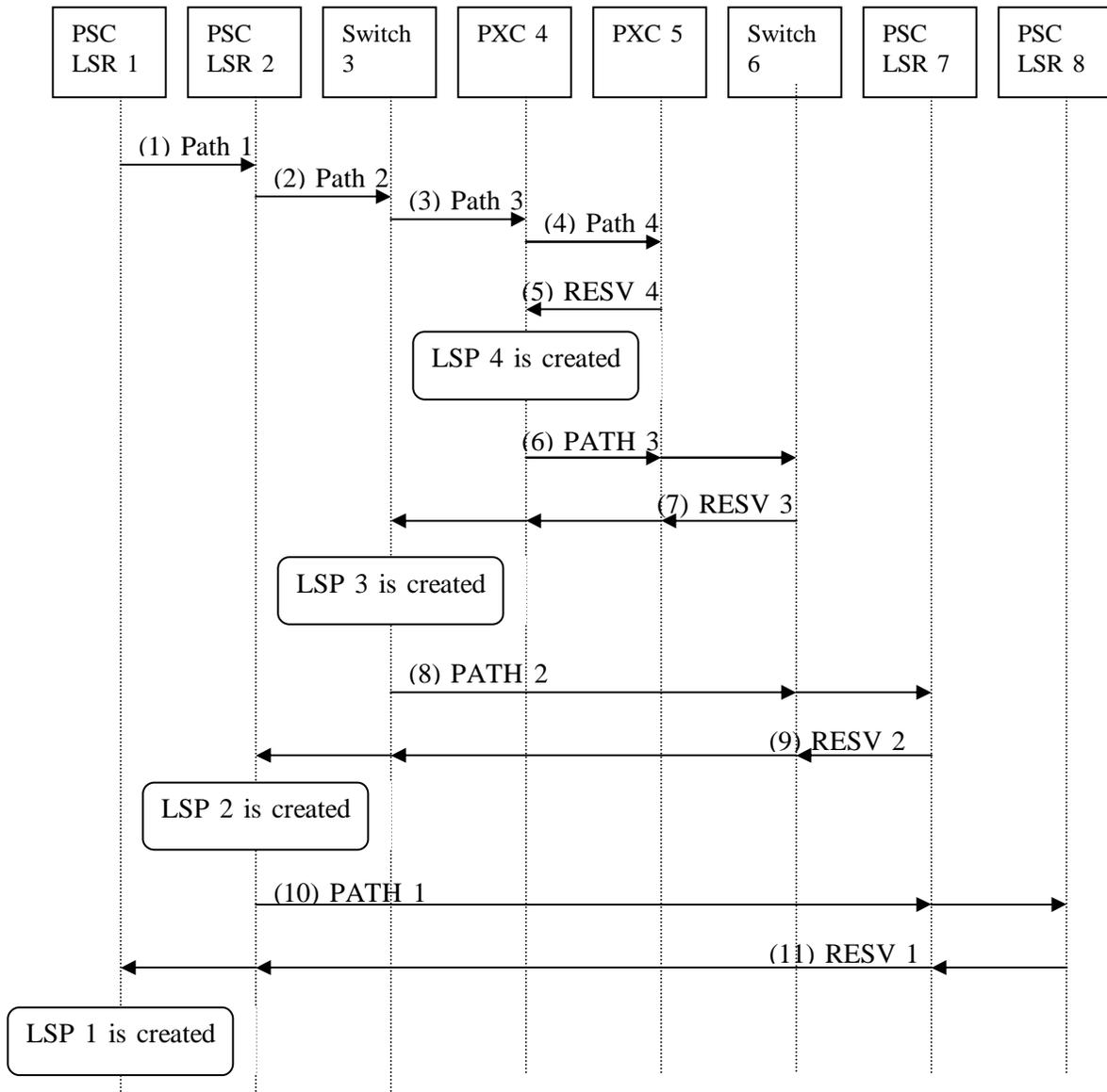
Figure 3.15: the time-sequence of establishing a hierarchical LSP
