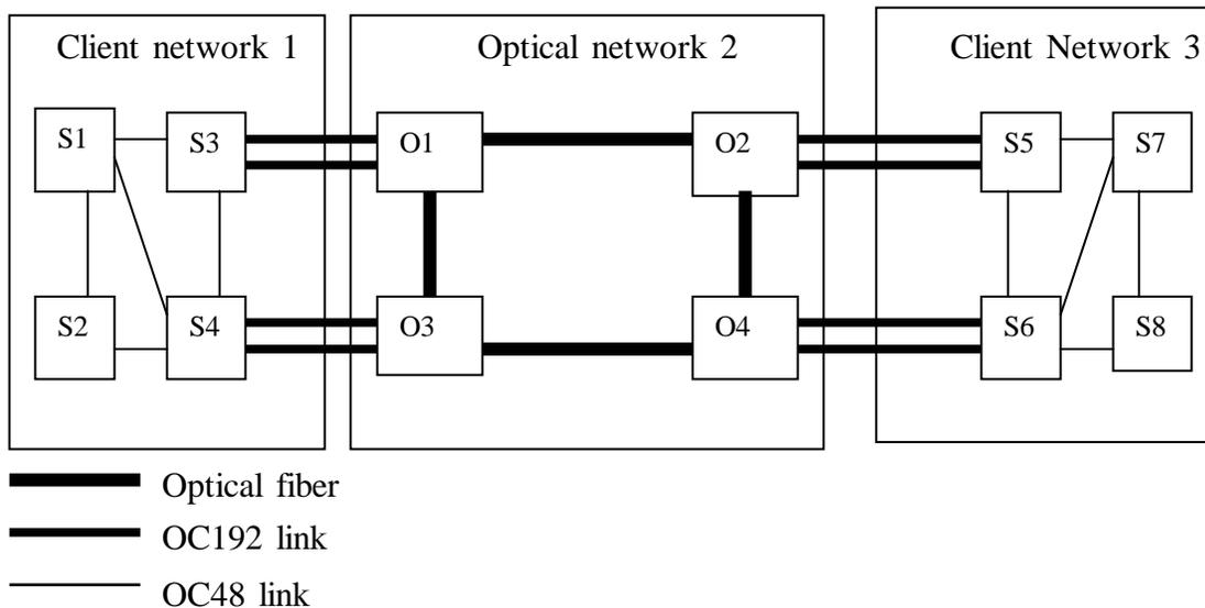
Figure 5.1: the network to show end-to-end 1:1 LSP protection
