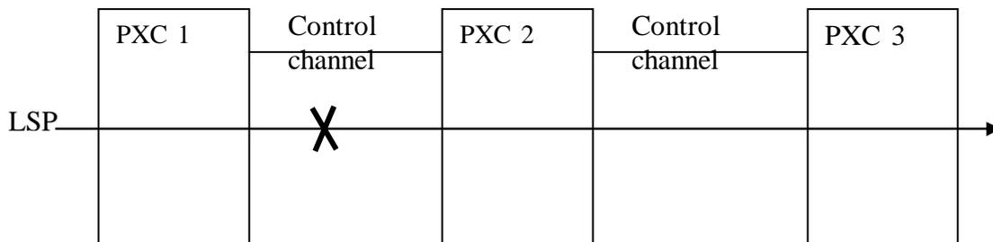
Figure 3.8: LMP fault management localizes the fault
