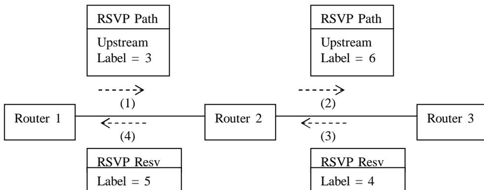
The forwarding entry in Router 2 for direction from R1 to R3
