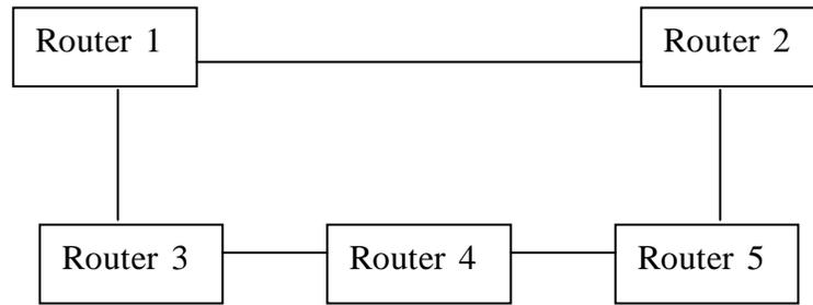
Figure 4.12: local reroute suffers packet loss for seconds
