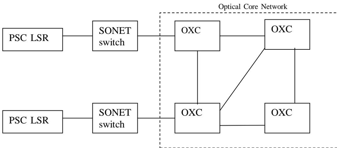
Figure 1.5: a GMPLS mesh network example
